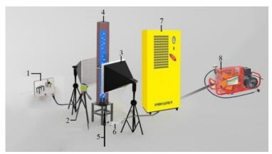
1-computer; 2-high speed camera recorder; 3-LED lamp; 4-simple flotation column; 5-bubbler; 6-gas mass flow meter; 7-flotation column console; 8-air compressor
